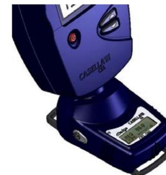
Switch on the CEL-110 calibrator. The *d*Badge will automatically recognise a calibration tone is present and enter the calibration mode, showing the screen below.
